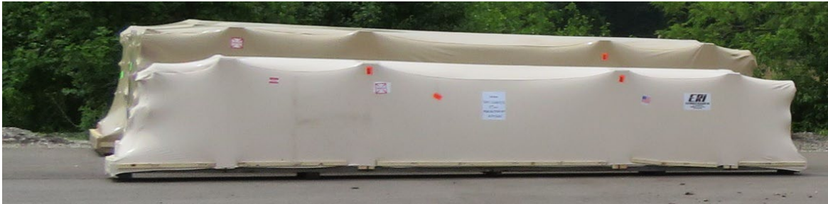
Heat Shrink Skid Tarps Provide Long Term Weather Protection
